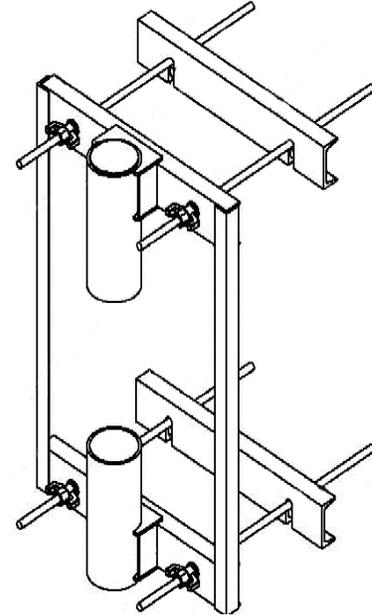
**Description** EZ-Link Double Connector for use with the SafeLink Horizontal Lifeline System. Attaches directly to rebar cage (6 #9 rebar or larger). Vertical post receptacle. All associated materials must be rated to meet OSHA, federal, state and local government regulations for fall protection anchor points.
